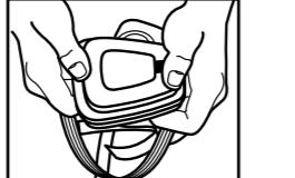
3. To replace the 5P71 (07194) filter, remove the 501 (07054) filter retainer by lifting on the tab as shown.
