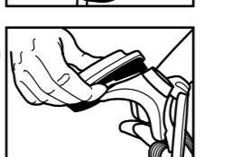
**NOTE:** Use of the 501 (07054) filter retainer may aid respirator wearer in conducting a negative pressure user seal check.
