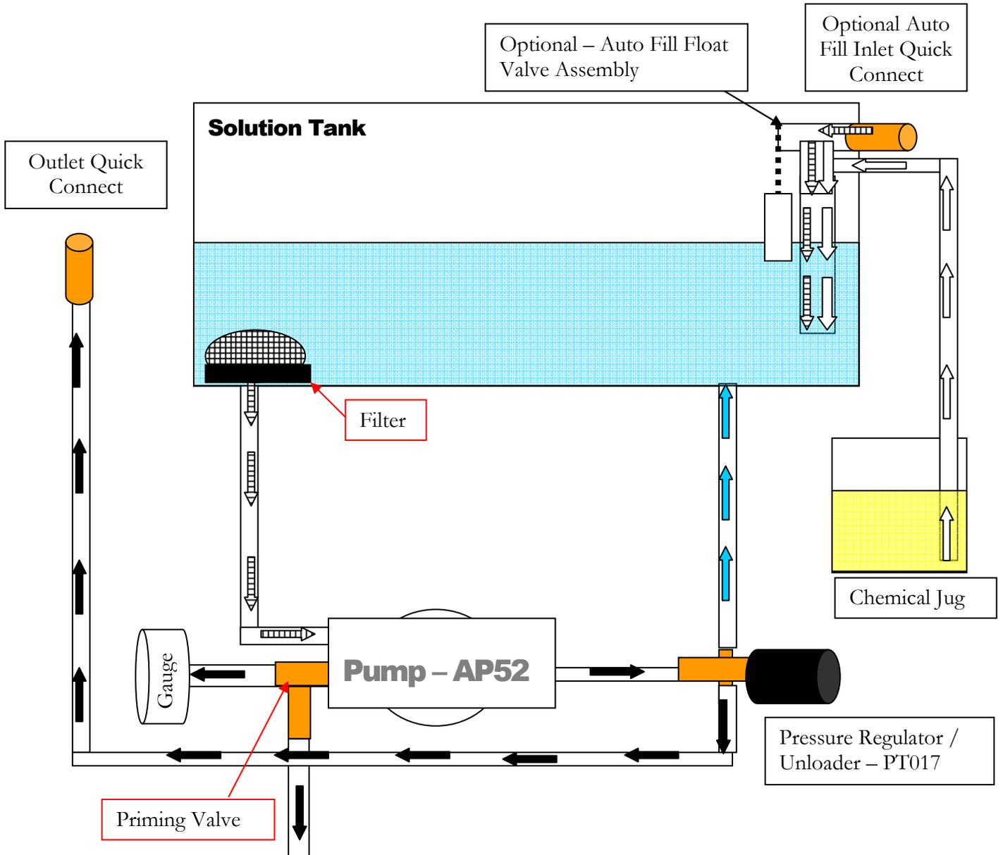
When Priming Valve held open water flows through hose to Recovery Tank
