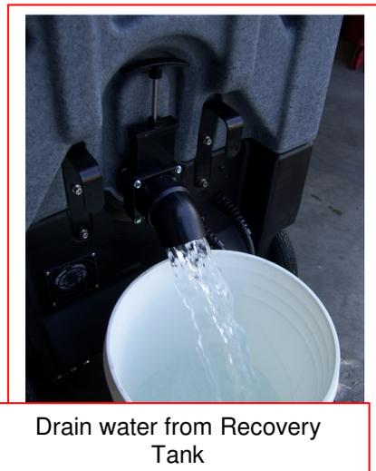
Drain water from Recovery Tank
