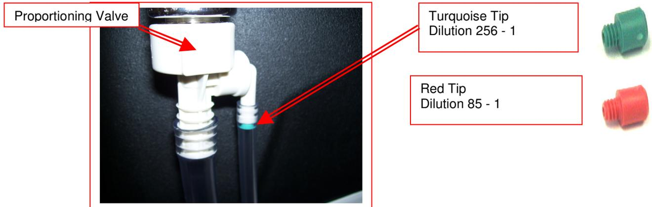
**Metering Tip Kit (Hydro-Force Item# PDE001)** contains 14 different colored metering tips, allowing dilution rates from 11:1 up to 427:1. Refer to the chart below to select the tip that meets the dilution rate for your chemical application.
