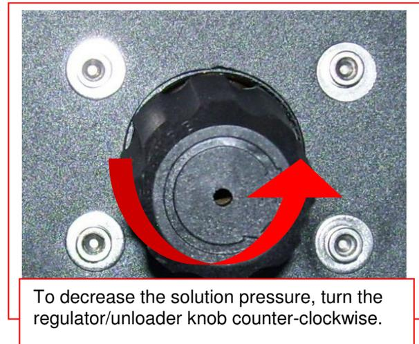
The maximum pressure setting is 500psi; however, the highest pressure attained is dependent on the amount of water flow at the tool:
