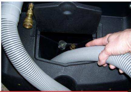
Vacuum acid solution out of Solution Tank
