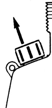
When pressurizing sprayer, read gauge as cap automatically rises. Recommended pressure is 25-40 psi (2-3 Bar)
