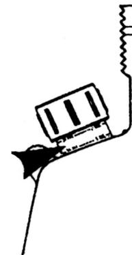
To release pressure in tank, pull pressure valve up until pressure is completely exhausted.
