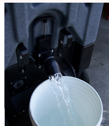
Drain water from Recovery Tank
