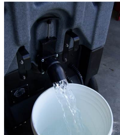
Drain water from Recovery Tank
