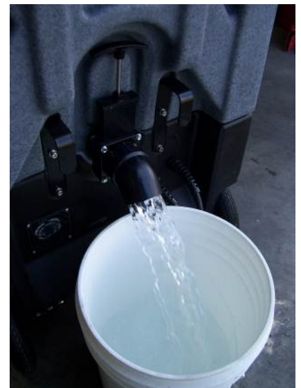
Draining the Recovery Tank
