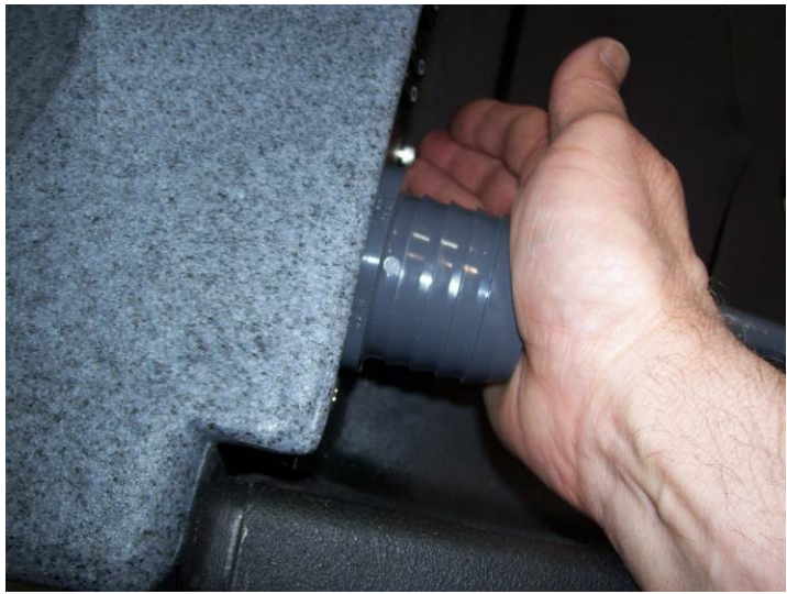
BLOCKING THE VACUUM PORT TO PRIME PUMP
