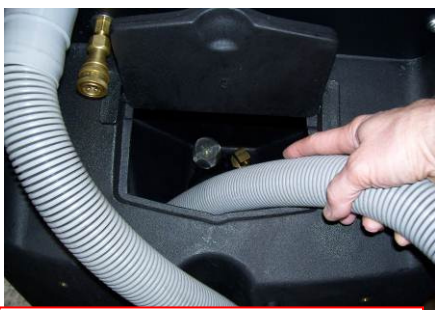
Vacuum acid solution out of Solution Tank
