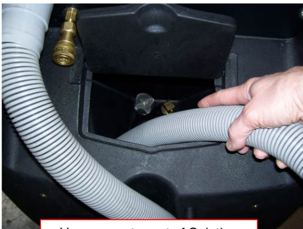
Vacuum water out of Solution Tank
