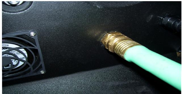
If not using the waste pump-out, the pump-out hose does not need to be connected. When the recovery tank fills during cleaning, the float assembly in the vacuum inlet filter will rise and will automatically shut off the vacuum air flow to prevent the recovery tank from overflowing and waste water from getting into the vacuums. When this occurs:
