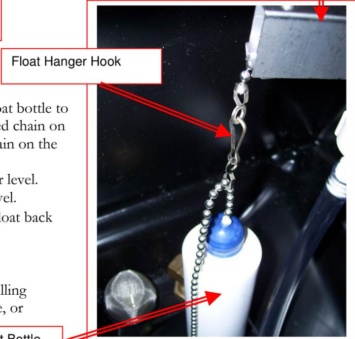
**To adjust the water level in the solution tank:**
