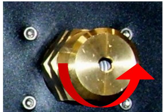
To decrease the solution pressure, turn the regulator knob counter-clockwise.
