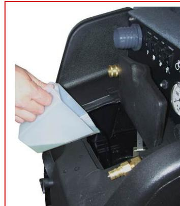
Add appropriate amount of chemical to water in solution tank
