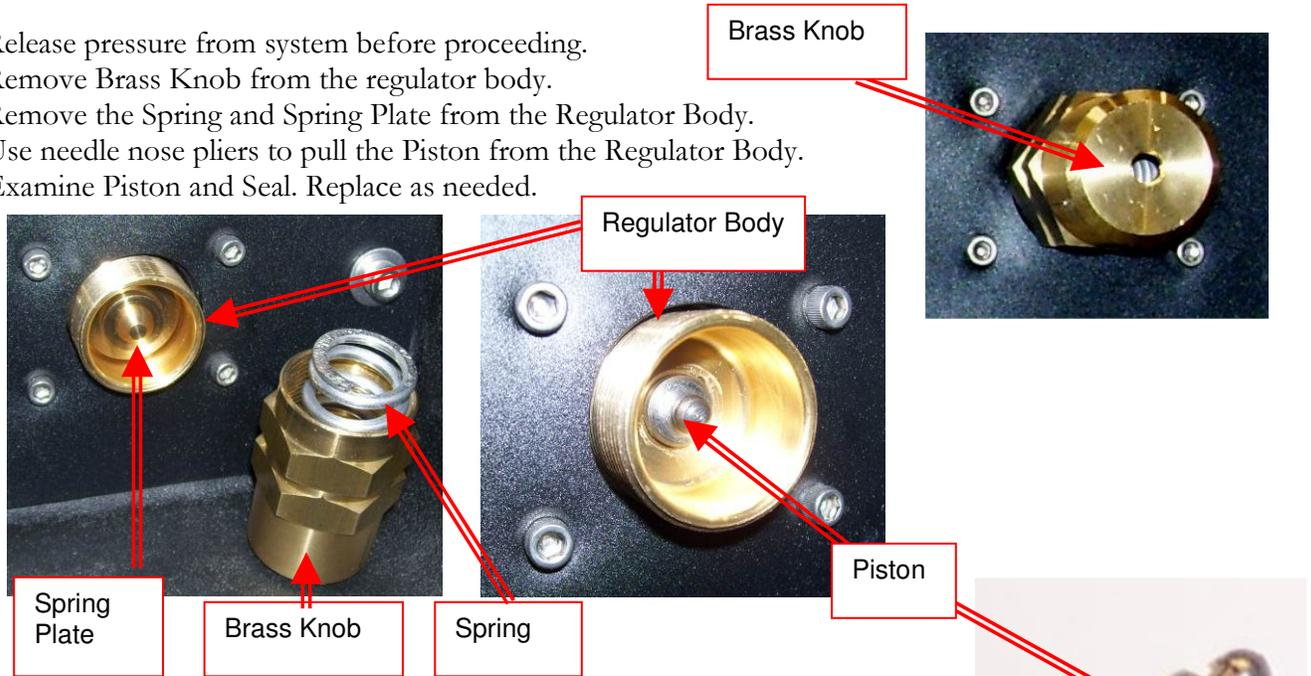
6. Use a synthetic grease with Teflon such as Ultra-Slick or Super-Lube to lubricate the seal on the regulator piston.
