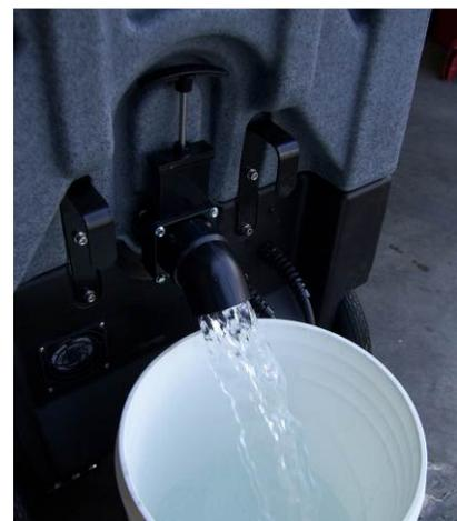
Drain water from Recovery Tank
