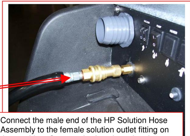
Connect the male end of the HP Solution Hose Assembly to the female solution outlet fitting on the machine. Connect the female end to the cleaning tool.
