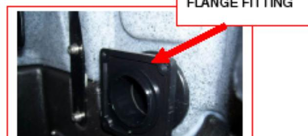
Unless damaged or leaking between tank and flange, the flange fitting does not have to be removed
