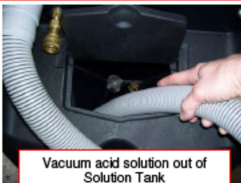
Vacuum acid solution out of Solution Tank
