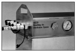
This system purifies, regulates, and distributes plant air to as many as four air-line respirator users. A sealed, rugged, stainless steel case prevents contamination of interior components. Using external controls, water condensa-
