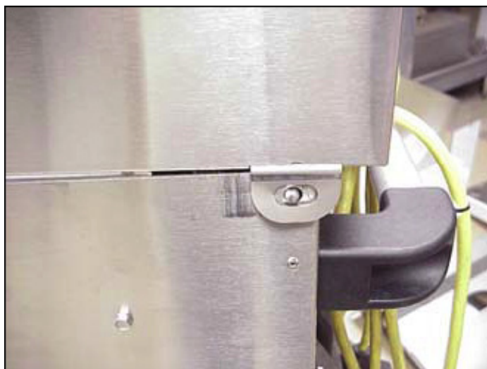
Figure 3: Solution slides forwards and engages clips on side of dehumidifier.
