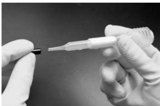
**Figure 3** Allow Air to Enter Bellows
