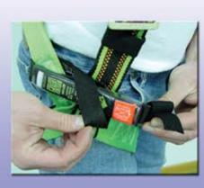
1. Mount to upper rear web strap by "choking" through loop (Be sure loop is past metal adjustments.)
