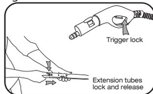
The steam gun has a trigger (ON) lock located just behind the trigger. This lock can be used for continuous steam without having to hold the trigger. To set the lock, push down the trigger, then while the trigger is down slide the lock to hold the trigger.
