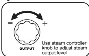
The flow rate of the steam emitted can be regulated by turning the steam controller and can be adjusted to the level required. Turn the controller knob clockwise to increase the steam output and counter clockwise to reduce the steam output. (Fig.3)
