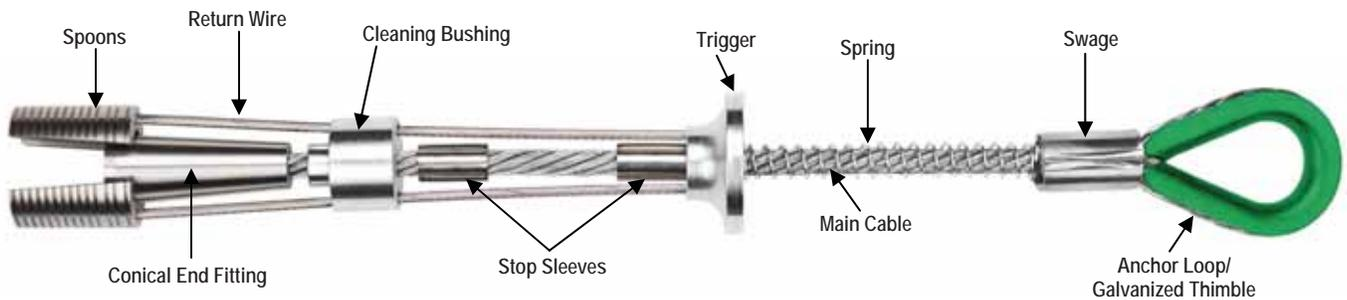
The Miller Grip Friction Bolt Anchorage Connector Model #494 is designed for:
