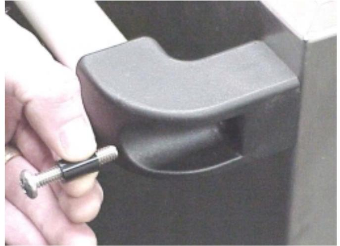
3. Place the nut retainers inside the back of the cabinet, as shown below. Using a Phillips screwdriver, thread a #10 x 5/8" screw through a nut retainer, the cabinet, and into the small boss on a handle bracket. Do not tighten completely.
