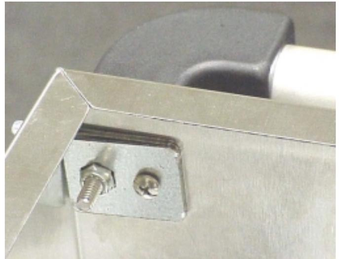
4. Insert the handle tube into the remaining handle bracket and into the attached handle bracket. Attach the second handle bracket as described above.
