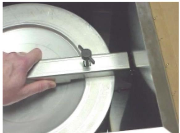
3. Disengage the screw and spacer from the hole in the front of the cabinet and remove the filter hold-down bar.
