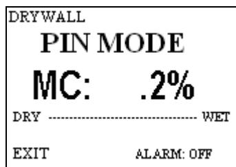
3. Push the contact pins into material to be tested. Any Delmhorst electrode may also be used in **DRYWALL** mode by simply attaching it to the connector next to the contact pins.
