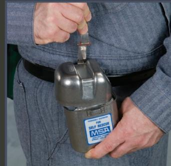
**4** Grip the red release lever between thumb and forefinger and pull up hard. This should break the seal and release the locking mechanism to loosen the cover.
