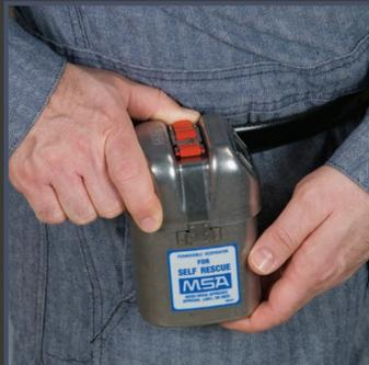
**2** Release the locking device by pressing the thumb under the red release lever and pushing up ...
