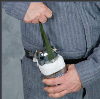
**6** Grip the head harness of the respirator, and pull the respirator out of the container. (If the container is dented, preventing release, see step 14.) Discard container.
