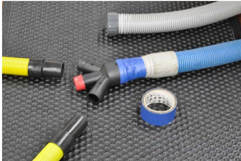
Temporarily attach the Main W with a HB300 (sold separately). Insert the barbed end into the end of 2" truckmount/portable suction line. If you do not have a HB300, use tape to temporarily seal the Main W to the end of the extraction line.
