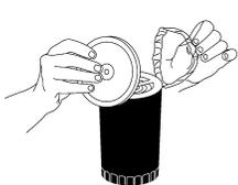
Turn off machine. Lift off cartridge lid & discard clear film liner. Cartridge life is rated at 270 hours.
