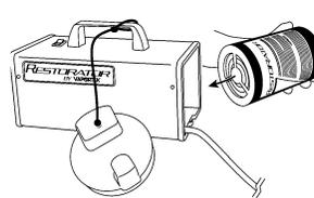
Insert open end of cartridge into back of machine, seating firmly against internal gasket. If substantial oil leakage is evident, do not use.
