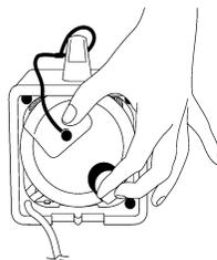
Install spring-loaded cover plate against cartridge lid & twist to lock into place.
