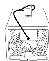
To operate, plug cord into power outlet. Always unplug Restorator before removing cartridge. The cord can be coiled for storage in the back of the rear cover plate.
