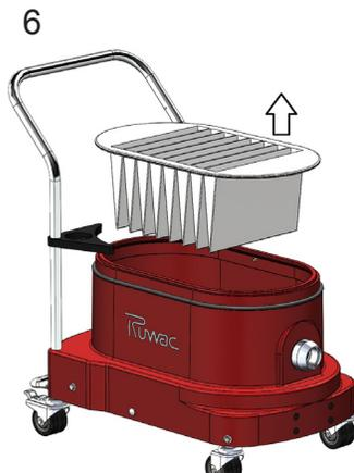
Replace filter as required or if the filter shows signs of staining, tears or holes. (See pg. 6 for instructions)
