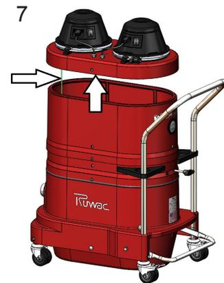
Replace the motor deck, and attach the ground wire.
