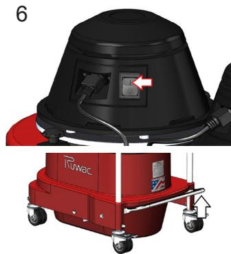
6 Release the dustpan, and turn the machine ON / (I).
