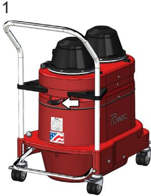
With machine off, knock material off the filter via the manual shaker by moving it in and out rapidly for 10 seconds.
