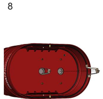
8 For WS motordecks, pinch and insert brackets into the vacuum inlets into the vacuum inlets on the bottom of the motordeck.
