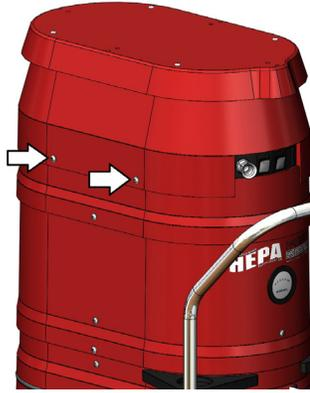
Disconnect hood from motor deck by removing 4 screws.
