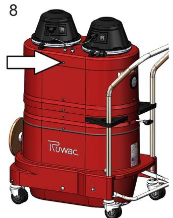
With the motor running and inlet blocked, secure the motor hardware.
