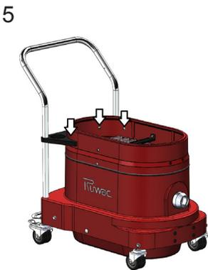
Remove the handle bar bracket screws.
