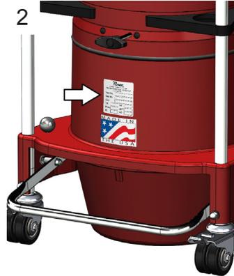
2 Connect the machine to the proper power source, as indicated on the machine's serial tag.
