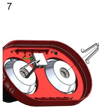
7 For WNS motordecks, pinch and insert the brackets into the bottom of the aluminum motorheads.
