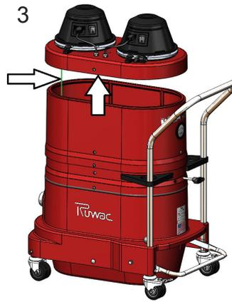
Remove the motor deck and disconnect the ground wire.
