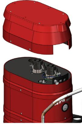
Remove silencer hood from motor deck.
