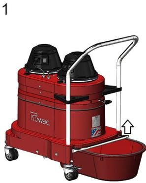
1 Pull up on the dust pan lever to release the dustpan. Check that the dustpan is completely empty then replace.
