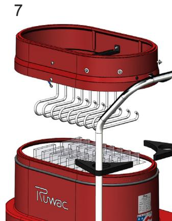
Remove the filter cage housing spacer assembly.
