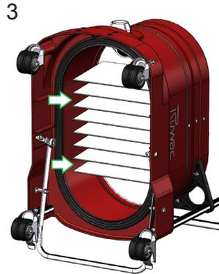
Lock the rear casters. Carefully tip the machine back onto the push handle in order to inspect the filter.
