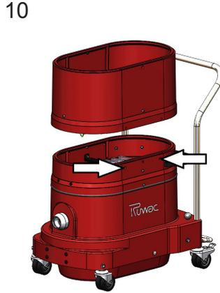
Lift the HEPA Maxx module and drill out holes with a 1/2in bit. There are two locations on each side.
