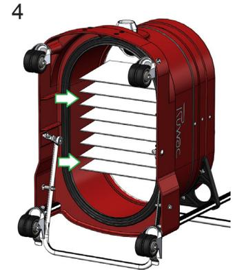
Remove any material between the pleats, by hand only. Inspect the pleats of the filter for tears and material blockage; Inlet for wear.
