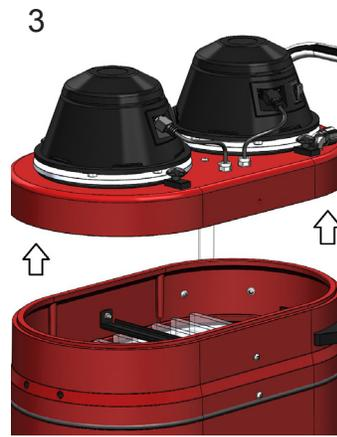
Separate and remove the motor deck from the housing.
