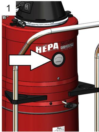
To ensure optimal performance of the HEPA Maxx filter, replace when the head loss reaches 8 inches of water column.
