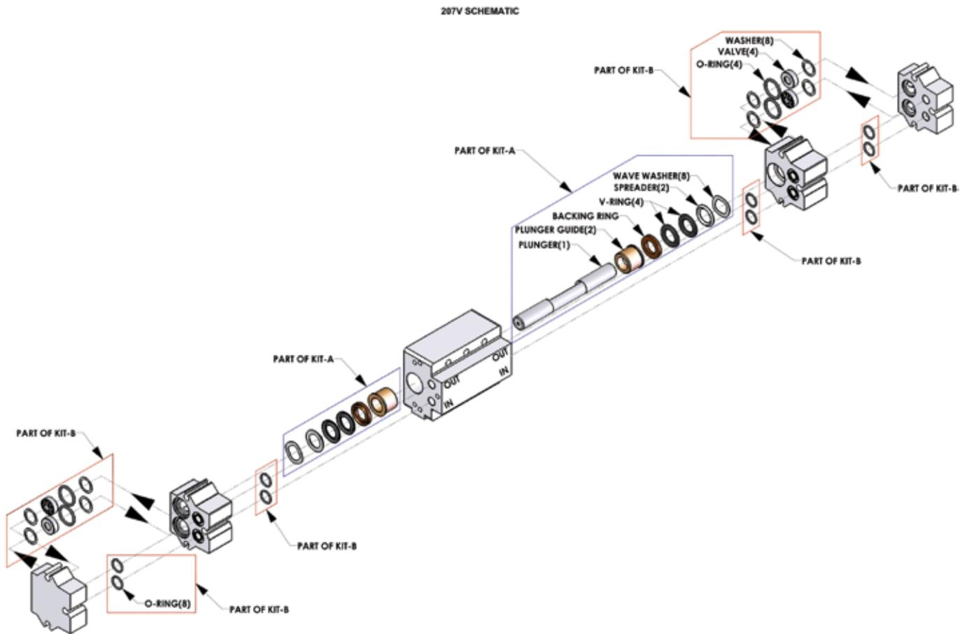
Repair Parts illustration for Plunger Pump
