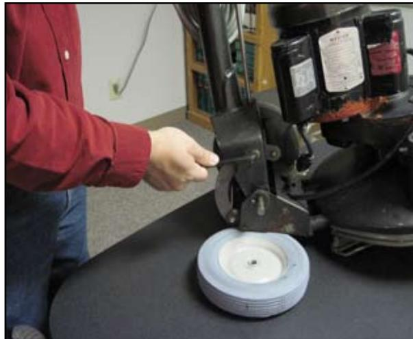
**Figure 6-9. Tighten Setscrew**
