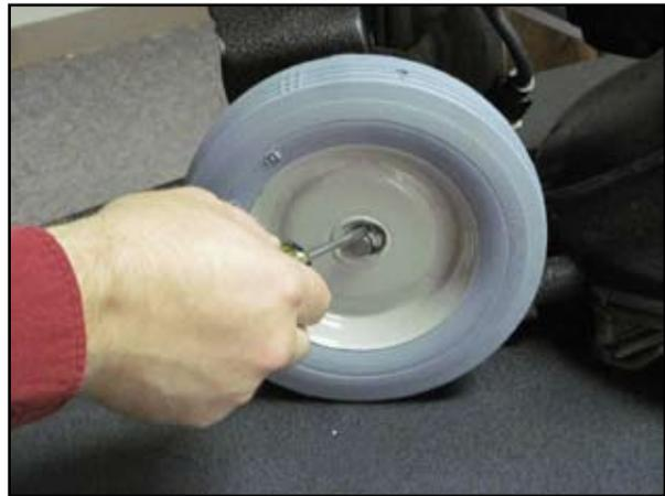
**Figure 6-8. Remove Retaining Clip with Screwdriver**
