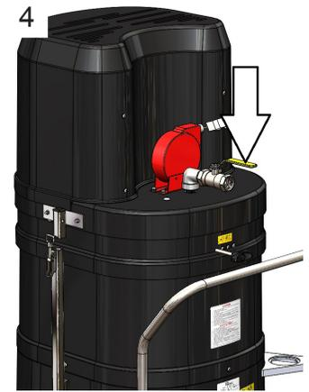
To turn off the machine, close the ball valve by turning the lever away from you
