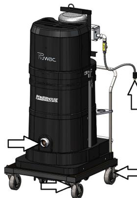
Also check for continuity between the plug and inlet, all four casters, and frame hardware if applicable.
