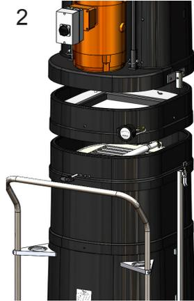
Release the clamps and remove the motordeck using a hoist
