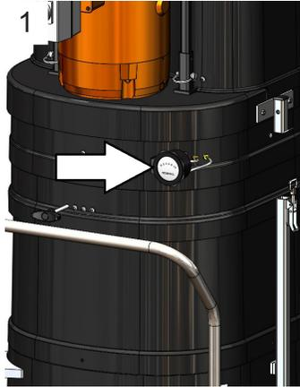
To ensure optimal performance, replace the filter at 8" W.C.
