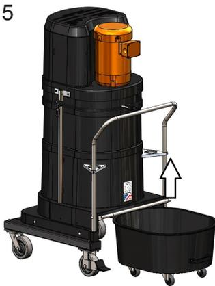
5 Empty the dustpan by releasing the rear lever.
