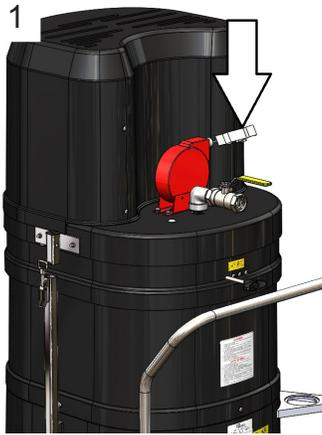
If included, affix the retractable grounding cable to an adequately grounded object
