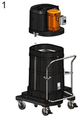
Remove the motordeck using a hoist.
