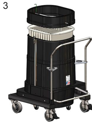
Lift the filter ring and remove the filter from cage.
