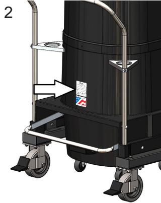
2 Connect the machine to proper power source, as indicated by the serial tag.
