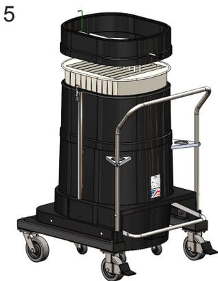
Place the filter ring back onto the base. Be sure that the filter is seated properly.
