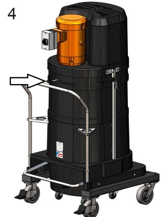
4 Use the filter shaker to clean the filter before and after each use.
