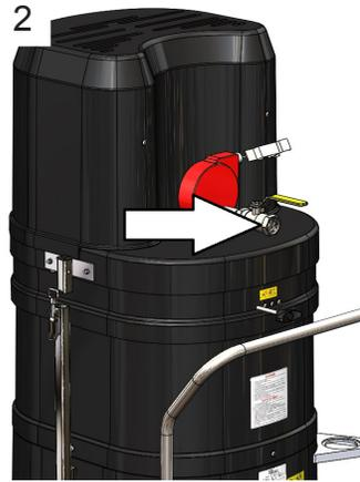
Attach a full port air supply connection. A 1" unrestricted air line is required for optimal performance
