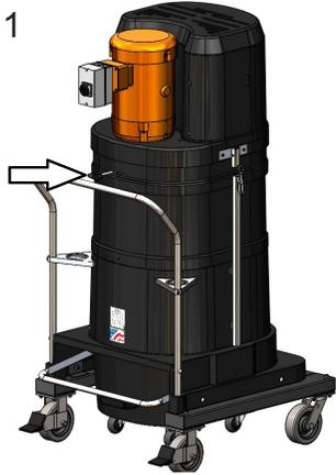
Use the shaker bar to clean the filter while the machine is off.
